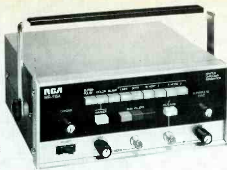
Fig. 1 Some features of the RCA Master Chro-Bar generator Model WR-515A include the usual patterns and color bars plus Blank raster, Superpulse, and a selectable number of dots and lines. Also, the patterns can be obtained as standard video, or modulating an IF carrier or a Channel 3 carrier.
